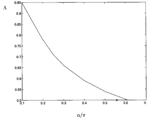
Figure 5. The singularity exponent  $\Lambda$  as a function of the angle  $\alpha$ , for  $\nu = 0.3$ . The result of Bažant and Estenssoro [5] is marked by \*.
