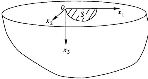
Figure 1. Surface-breaking crack in a half-space.
