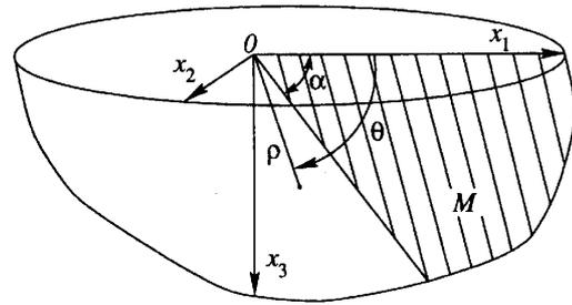
Figure 2. Crack geometry near the termination point  $O$ .
