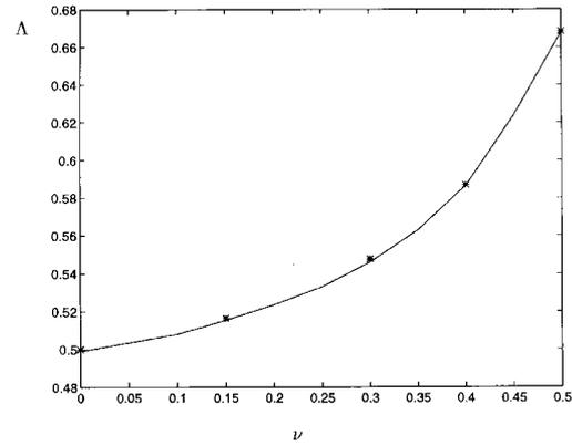
Figure 4. The singularity exponent  $\Lambda$  as a function of the Poisson ratio  $\nu$ , for  $\alpha = \pi/2$ . The results obtained by Benthem [1, 2] are marked by \*.
